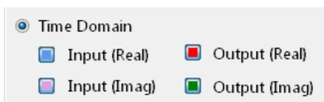
The signal generator automatically converts its output signal into a complex signal. The options **Real** and **Imag** refer to the real and imaginary components of the input and output signal respectively.
