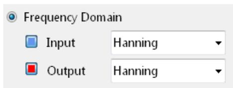
Two traces are used for the frequency domain analysis (as seen on the left). Although when **Transfer function estimation** is enabled, only the **Output** (red trace) is shown.
