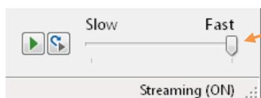
Signal generator playback speed (streaming only): You may adjust the chart update speed by setting the slider accordingly.
