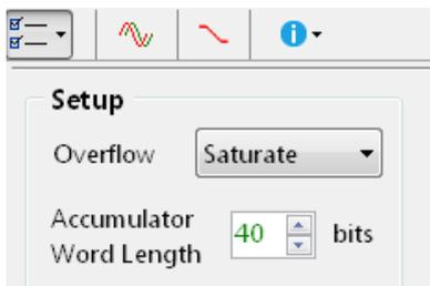
For fixed point implementations the tool allows designers to specify the overflow arithmetic rules as: Saturate or Wrap. Also, the Accumulator Word Length may be set between 16-40Bits allowing designers to quickly find the optimum settings to suit their application.
