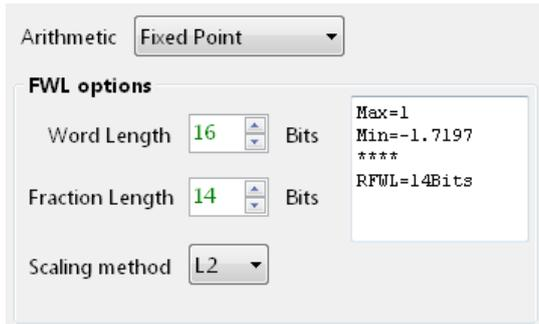
For the example considered herein, it can be seen that the tool summarises the maximum and minimum coefficient values obtained with double precision. As seen, a recommendation of 14Bits is given as the largest negative value is  $-1.7197$  which with a word length of 16Bits would require at least a fraction length of 14Bits.
