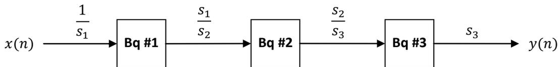
Figure 5 - biquad cascade scaling concept.
