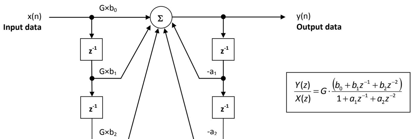
Figure 1 - Direct Form I (biquad) IIR filter realization.
