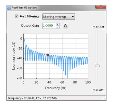
The ASN filter designer's signal analyser implements an extra post filter, H3. Unlike the H1 and H2 filters, the H3 filter is *always lowpass* and is preceded by an optional mathematical function operation (see above).
