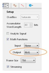
The fullwave rectification and  $\frac{1}{\sqrt{2}}$  mathematical operations can be summarised as one RMS () operation, i.e.  $\frac{abs()}{\sqrt{2}}$  and implemented via the Output Math Function in the signal analyser. This scaling trick is made possible as H3 is a linear filter (see post filtering), although this operation is equivalent to using abs () with an output Gain of 0.707.
